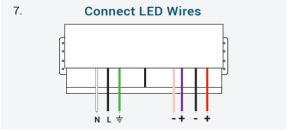
Connect wires on the driver to the respective wires on the LED light using an appropriate connector. Cap off the 0-10V dimming wires when not in use.
