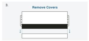
Lift the cover plate at the top of the power supply. This will expose the Input and Output wires.
