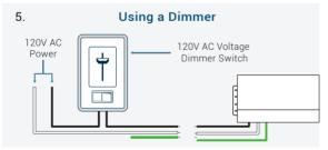
When using a 3-pole TRIAC dimmer as a single pole make sure to cap the additional line and connect the rest of the wiring as recommended by the dimmer instructions. Find our list of compatible dimmers below.
