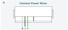
Loosen the Input Power L and N wires and attach the AC Live and Neutral wires respectively. If you are installing this with TRIAC/Phase Cut dimming, follow Wiring Diagram #1, and if you are using 0/1-10V dimming, please follow Wiring Diagram #2 (See page 7).
