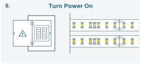
Turn the main breaker for the AC line back on to power your non-dimmable power supplies. The LED strip should turn on.
