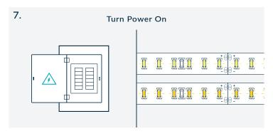
Turn the main breaker for the AC line back on to power your non-dimmable power supplies. The LED strip should turn on.
