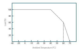
To extend the power supply's life, refer to the Derating Curve above and derate according to the ambient temperature
