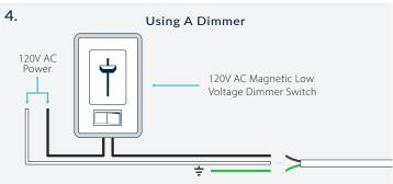
Connect the AC line ground (G) to the green wire from the Power Input Wire. Do the same with the AC neutral wire to the white wire on the driver and the AC live wire to the black wire. you can secure these connections with a terminal block.
