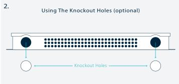
It can be mounted in any orientation, the chosen location must be able to support the weight of the power supply with 12" of clearance for proper ventilation. Never mount it next to objects radiating heat.
