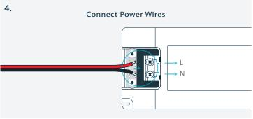
Unscrew the left and right cover plates on the power supply. This will expose the Input and Output Power Terminals.
