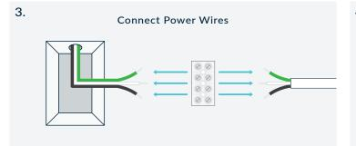
Connect the AC line ground (G) to the green wire from the Power Input Wire. Do the same with the AC neutral wire to the white wire on the driver and the AC live wire to the black wire. you can secure these connections with a terminal block.
