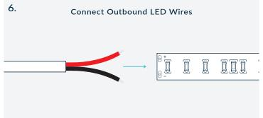
Connect the driver's Output Power negative (-) wire to the - channel on the LED strip. Connect the positive (+) wire to the + channel.
