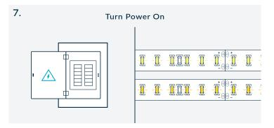
Turn the main breaker for the AC line back on to power your non-dimmable power supplies. The LED strip should turn on.
