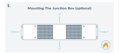
It can be mounted in any orientation, the chosen location must be able to support the weight of the power supply with 12" of clearance for proper ventilation. Never mount it next to objects radiating heat.
