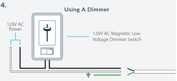
When using a 3-pole dimmer as a single pole make sure to cap the additional line and connect the rest of the wiring as recommended by the dimmer instructions. Find our list of compatible dimmers below.
