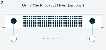
Remove wiring knockouts as needed and install 3/8" romex connectors or bushings to reduce strain on wires. One set of knockout holes is reserved for input voltage while the second set is reserved for output voltage.
