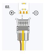
Double check the polarity of the strip to match the positive (+)markings together and negative (-) markings together. If you accidentally close the connector before you're ready, you can use a small flathead screwdriver to pry the top back open.
