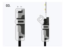
Open the top of the grip connector and insert the LED strip inside. Make sure the LED strip is facing up towards the translucent top and the solder pads are directly above the small hooks on the connector.
