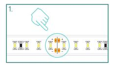
Find the cut line on the strip (between the solder pads).
