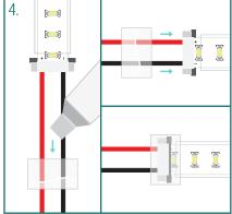
Fill the end cap (with holes) with sealant and slide carefully over the connector at the end of the strip.
