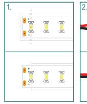
Cut the strip and remove the silicone covering just enough to expose the solder pads on the strip.
