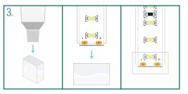
Fill an end cap (without holes) with sealant and slide it over the end of the strip until it fits snugly.
