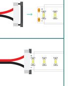
Carefully insert the strip into the connector and ensure it fits snugly.
