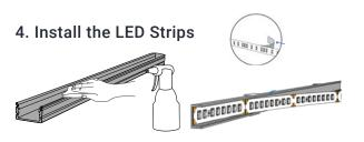
Clean any dust or dirt from the aluminum channels. Use rubbing alcohol or alcohol pads for optimal results. Insert the strip light into the channels by peeling the cover of the 3M tape backing a few inches at a time, while gently pressing the strip light to the channel. Ensure that the strip light is snugly fitted into the channel, so it won't fall out.
