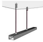
Please keep in mind that the cable is non-conductive of power. Run power wires parallel to the pendant cable as needed.
