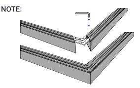
Some aluminum channels come with channel connectors. To install the aluminum channels using the channel connectors simply slide the channel connectors into the grooves on the back of the aluminum channel and use the black set screws to secure the channel connectors in place. It is easier if you secure the channel connectors on one channel first and continue with the other..
