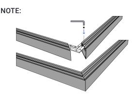
To install channel connectors simply slide the channel connectors into the grooves on the back of the aluminum channel and use the black set screws and secure the channel connectors in place using a hex tool. It is easier if you secure the channel connectors on one channel first and continue with the other.
