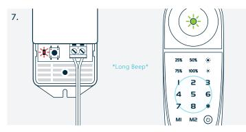
Press the black sync button on the receiver once. - The Power Indicator LED will remain static- then quickly press and hold the zone you wish to assign that receiver to (1-8) on the remote. The Power Indicator LED on the receiver will flash faster, you'll hear a long beep and the Sync Status Indicator Light on the remote will flash 3 times. This indicates that the 2 devices have been synced.
