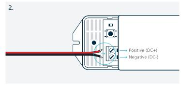
Loosen the Power DC+ and DC- screws and insert the black wire from your low voltage non-dimmable power supply in the DC- channel and secure the screw. Then insert the red wire from the power supply in the DC+ channel and secure the screw.
