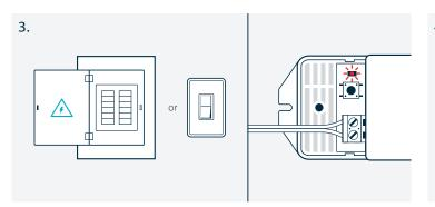
Turn the main breaker for the AC line back on to power your non-dimmable power supply. The red Power Indicator LED will turn on.
