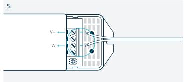
Loosen the Output V+ and any of the W screws (leave the other channels closed). Then connect the + wire from the LED strip to the V+ channel in the receiver and secure the screw. Do the same to match the negative (-) wire to the "W" channel.
