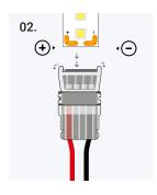
Check the polarity of the strip to match the positive (+) markings together and negative (-) markings together. If you accidentally close the connector before you're ready, use a small flathead screwdriver to pry the top back open.
