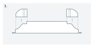
Unscrew the left and right cover plates on the receiver. This will expose the Input and Output Power Terminals.
