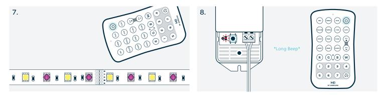
Press the Power Button on the remote control, the LED strip will turn on. Press the black Sync Button on the receiver once and the the Power
