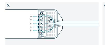
Loosen the Output V+, R, G, B, and W screws. Then connect the + wire from the LED strip to the V+ channel in the receiver and secure the screw. Do the same to match the rest of the letters to their respective channels.
