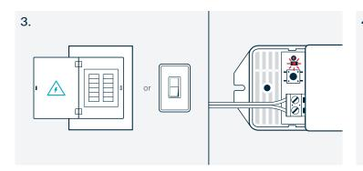
Turn the main breaker for the AC line back on to power your non-dimmable power supply. The red Power Indicator LED on the receiver will start flashing slowly demonstrating that it's getting power.
