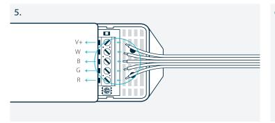
Loosen the Output V+, R, G, B and W screws. Then connect the + wire from the LED strip to the V+ port in the receiver and secure the screw. Do the same to match the rest of the wires to their respective ports R, G, B, and W.
