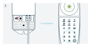
Press the black Sync Button on the receiver once and the the Power Indicator LED will remain static, then quickly press and hold the zone you wish to assign that receiver to (1-8) on the remote. The Power Indicator LED will flash faster, you'll hear a long beep and the Sync Status Indicator Light will flash 3 times. The remote is synced. You can assign unlimited receivers to a single zone (1-8) by syncing as many receivers as you need to the same number.
