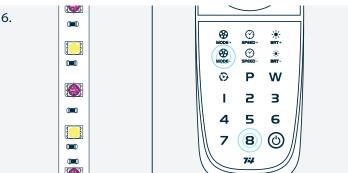
Press the Power Button on the remote control, the LED strip will turn on. Then hold Mode- and 8 simultaneously for about 2 seconds to go into the Zone Control Program, this will let you sync unlimited receivers into 8 independent zones. \*\*Pressing Mode+ and 8 will let you control unlimited receivers simultaneously with the Sync Control Program.
