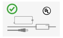
To meet UL requirements, only install with a Class 2 DC Constant Voltage LED driver.
