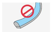
The Lucid™ LED Neon Strip Light is a side-bending LED strip light, which means it only bends in the opposite direction of the light, so bending it up and down will damage the LED strip light.
