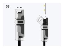
Open the top of the grip connector and insert the LED strip inside. Make sure the LED strip is facing up towards the translucent top and the solder pads are directly above the small hooks on the connector.
