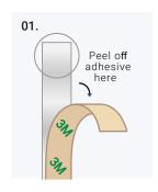
Remove 1/4" of 3M adhesive tape on the back from the end of the strip that you want to connect. It must be removed to allow it to fit properly with the solderless connector.
