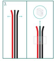
Spread the wires on the connetor and slide them through the hole in the end cap.
