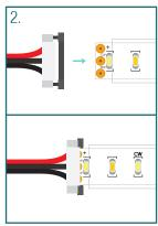
Carefully insert the strip into the connector and ensure it fits snugly.
