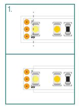
Cut away a small portion of the silicone sleeve to access the solder pads you will be connecting to.
