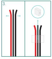
Spread the wires on the connetor and slide them through the hole in the end cap.
