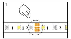
Find the cut line on the strip (between the solder pads).
