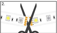
Carefully cut the strip on the cut line.
