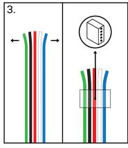
Spread the wires on the connector and slide them through the holes in the end cap.
