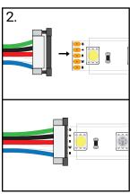
Carefully insert the strip into the connector and ensure it fits snugly.
