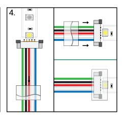
Fill the end cap (with holes) with sealant and slide carefully over the connector at the end of the strip.
