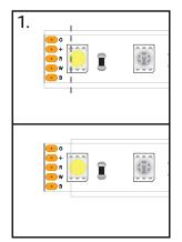
Cut the strip and remove the silicone covering just enough to expose the solder pads on the strip.
