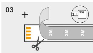
03 Remove 2" of the adhesive tape and its backer from the back of the LED Strip light.
