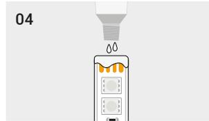
04 Apply Silicone sealant liberally inside of the silicone sleeve until ensuring it is completely sealed.
