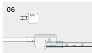
06 Grab the white plastic part of your connector and push the metal contacts through the window of the transparent case. Adjust it with pliers until you hear a click, and then let the sealant cure according to its own instructions.
