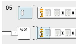
05 Slide the transparent case of your Outdoor IP65 Grip connector into the sleeve, until making sure that the strip is making proper contact.
