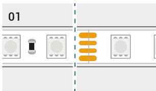
01 Cut the LED strip light and the silicone sleeve on the cutting point you want to install the connector. Keep in mind that for the Outdoor (IP65) ColorBright™ RGB 600 LED strip, you will need to cut both solder pads so that the piece to be attached to the connector has more surface area to insert into the connector head.
