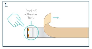
Remove about 1/4" of the paper backing and push back the adhesive at the tip of the LED strip where the connector will go to make enough room for it to fit. You can do this with a small blade or your own fingernails.
