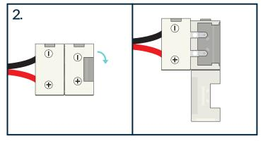
Open the connector lid as shown on the diagram above. You may need to use your fingernail or a small blade to open the latch.
