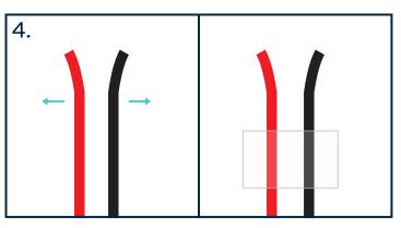
Separate the wires on the connector and slide them through the holes in the end cap (you can poke holes in it if needed).
