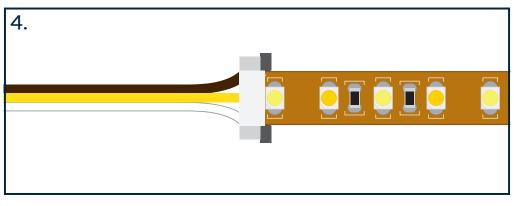
Test your LED strip by connecting it to the receiver placed between the strip and the low voltage power supply. Make sure you follow the positive (+) channel on the LED strip throughout your setup.
