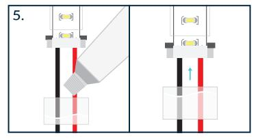
Test the connection by lighting the strip with a low voltage power supply. Once sure the connector works correctly, completely fill the the end cap with silicone sealant and slide down to cover the connection.
