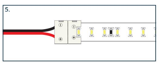
Now test the strip. If everything is connected properly and the polarity between the LED strip and the power supply is aligned then the LED strip will light up.
