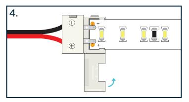
Check that the polarity of the strips match the polarity of power supply and then close the lid until you hear a snap. If the lid does not close fairly easy, make sure the notch and the first LED chip are aligned correctly.
