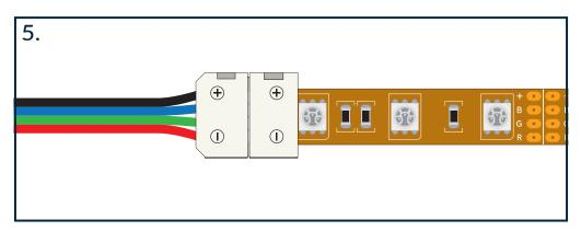
Now you can test the strip by providing 12 or 24VDC depending on the voltage of your LED strip. You can use the controller and the receiver placed between the power supply and LED strip for testing. You can also simply connect the positive wire from the power supply to the strip and check each negative color wire individually with the negative wire from the power supply. If everything is connected properly, the LED strip should light up.
