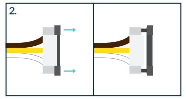
Pull the tray to the out position so the LED strip can be inserted. Be careful to not pull too hard as the trays are fragile and will break.
