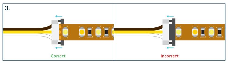
With the black tray in the out position, insert the LED strip as far as it will go, then simply push the black tray back into the in position to lock it. Make sure the connector is not upside as indicated in the diagram above.
