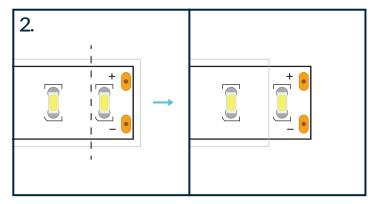
Trim the silicone sleeve to expose the tip of the LED strip where the connector will go. Be sure to measure how much you are trimming off so the end cap covers some of the sleeve.
