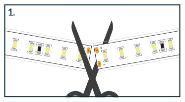
Use a sharp wire cutter or scissors to cut the LED strip along the cut marks that are found every 1" to 8" depending on the series you are working with. (Do not cut anywhere else except on the cut marks).
