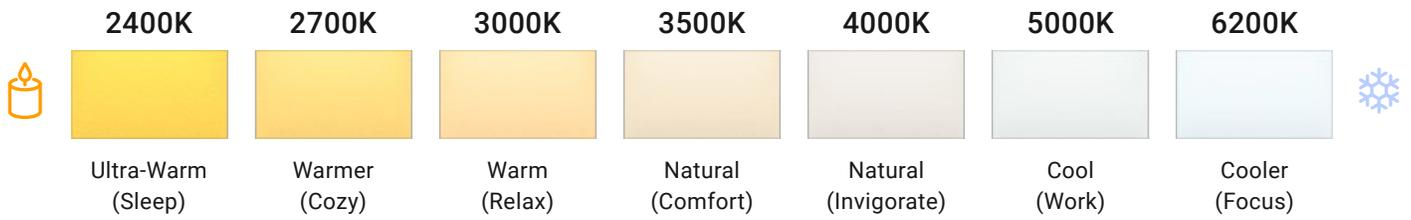
White lights are measured by the Kelvin Scale (K), which is an indicator of heat. When a metal is burnt at different temperatures, it changes color tone. This color changing process is a constant that is used in the lighting industry to indicate the tone of a white.
