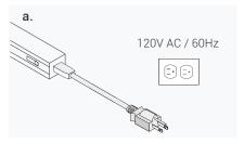
If you are going to plug your fixtures into an outlet, attach the 6 foot long Endeavor™ Plug-and-Play Power Cable (sold separately) to the Endeavor™ 120V Cove Light to power the fixture using an existing 120V AC outlet.
