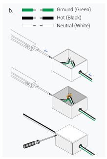
If you are going to hardwire your fixtures, attach the 6 foot long Endeavor™ Hardwire Power Cable (sold separately) to the Endeavor™ 120V Cove Light to hardwire the fixture directly to 120V AC. Then, insert the wires into the Endeavor™ Junction Box for hardwired installations and secure the connections with wire nuts. Use a head screwdriver to screw the top cover of the junction box to secure it.
