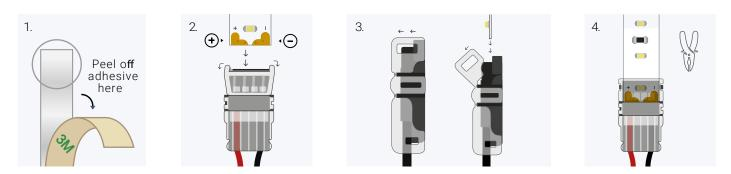
**1.** Remove 1/4" of 3M adhesive tape on the back from the end of the strip that you want to connect. It must be removed to allow it to fit properly with the solderless connector. (See Diagram 1)
